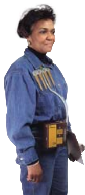
Clip holder to worker and pump to belt.
