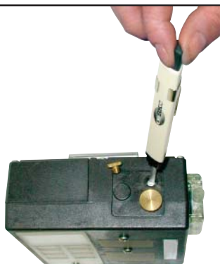
For low flow, turn valve screw counterclockwise.
