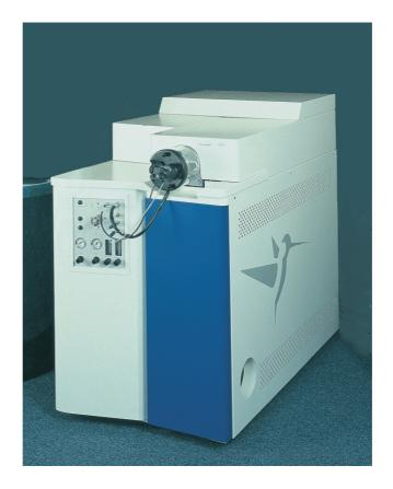
The Q-Tof 2 hybrid quadrupole time of flight mass spectrometer is available with electrospray ionisation (ESI) and atmospheric pressure chemical ionisation (APcI).
