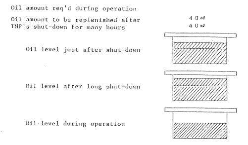
Oil replenishment: Detach oil sump in the way illustrated below, and replenish oil as required.
