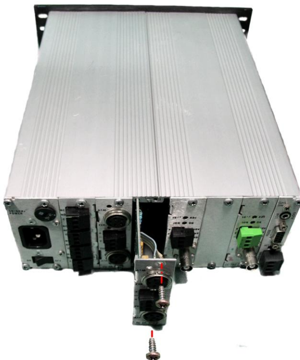
Fig. 3.3 - Removal / Installation of Modules
