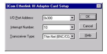
The card goes on the ISA number 0 bus. Cancel out of this screen if everything is correct. Next Select Protocols for the Etherlink III adapter. You should get this box. For LCQ communications we must have NetBEUI and TCP/IP. Other protocols used by the customer's network may be listed.
