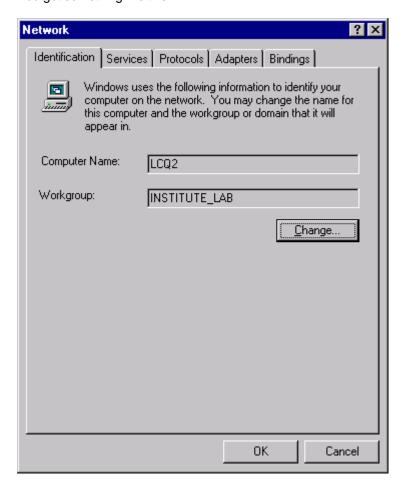
Select Adapters. You should get this box. The Etherlink III card is the one that Finnigan assigns to the LCQ. The Etherlink XL is for the customer's network.
