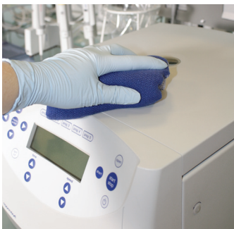
Figure 2: Wipe outside of centrifuge and clean rotor chamber and rotor with moist cloth and neutral detergents.
