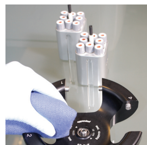
Figure 3: Decontamination of centrifuge, rotor and rotor buckets.
