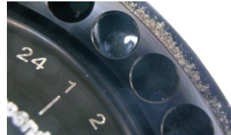
Figure 1: Localized corrosion in bore hole
