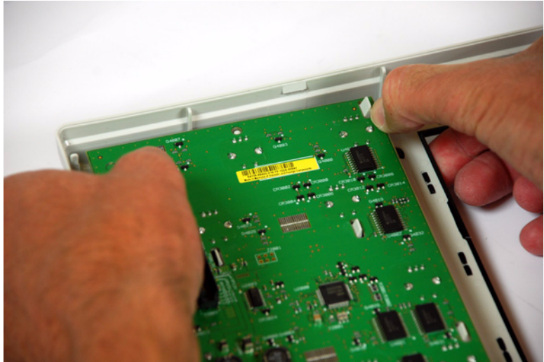
Figure 41 Removing the keyboard
