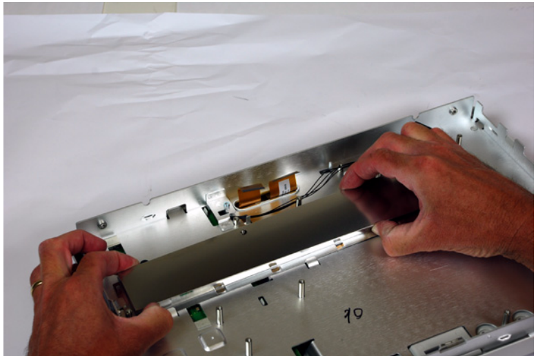
Figure 34 Removing the keyboard cable shield
