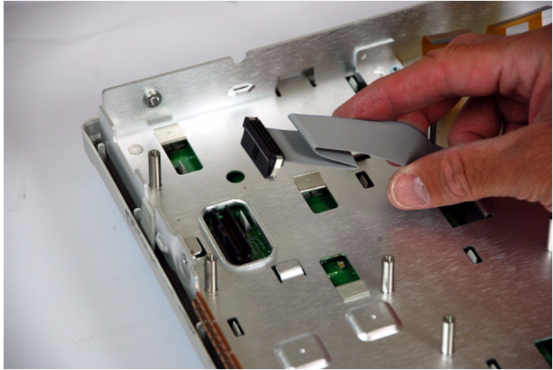
Figure 35 Disconnecting the keyboard cable
