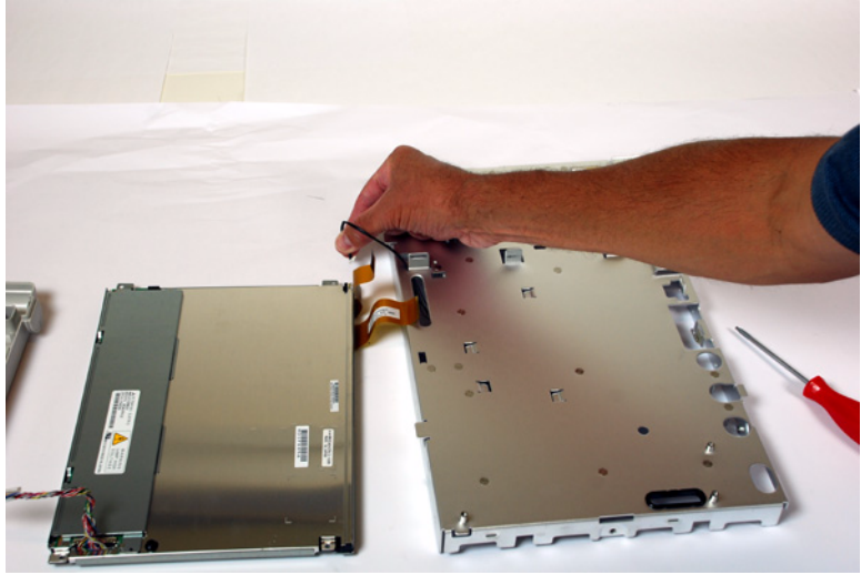
Figure 39 Disconnecting the backlight power cable
