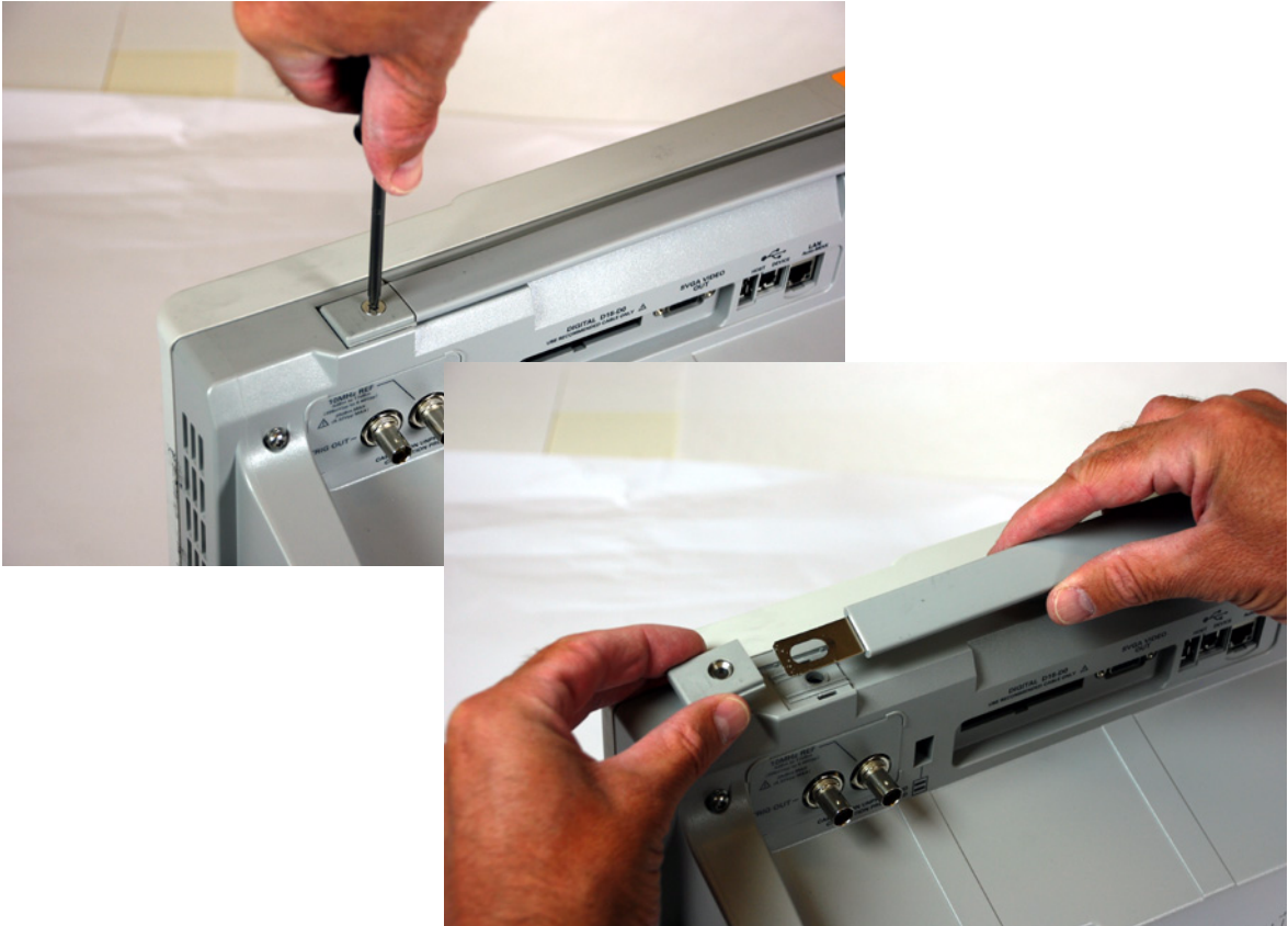
Figure 20 Removing the handle
