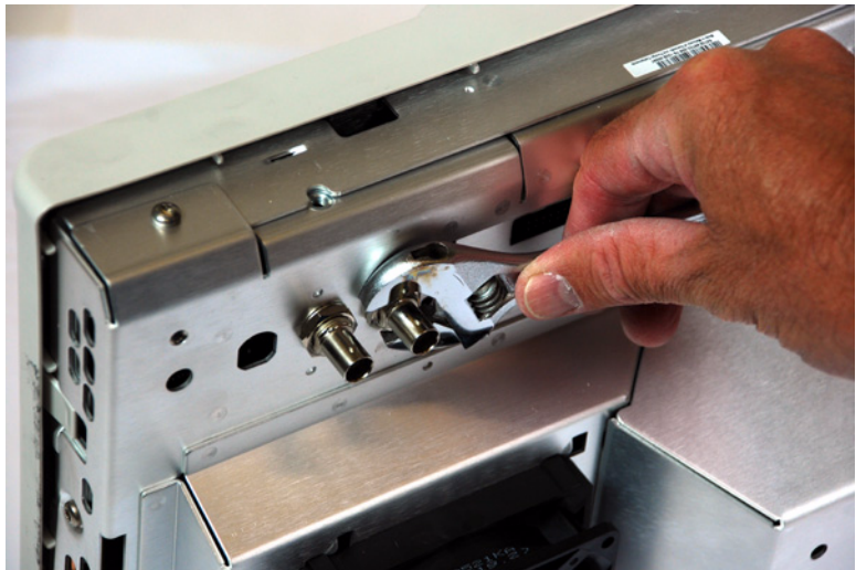
Figure 23 Removing the BNC securing nuts and washers
