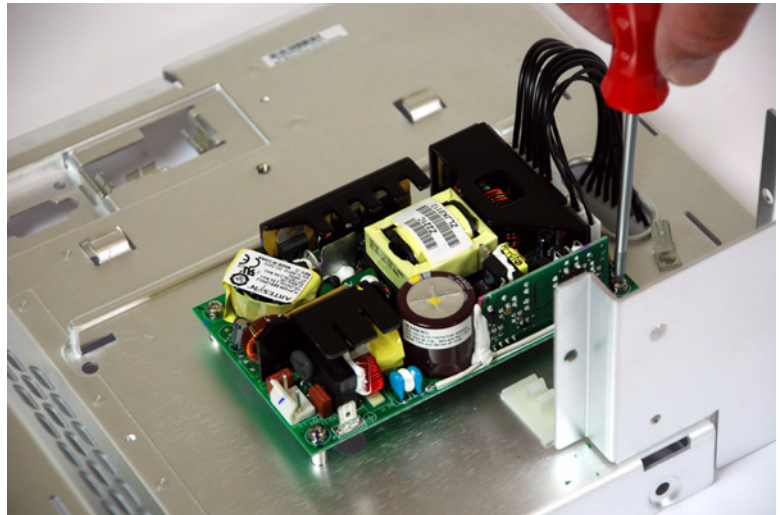
Figure 52 Removing the power supply
