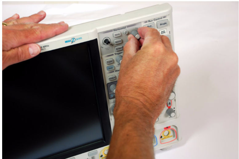
Figure 33 Removing the front panel knobs
