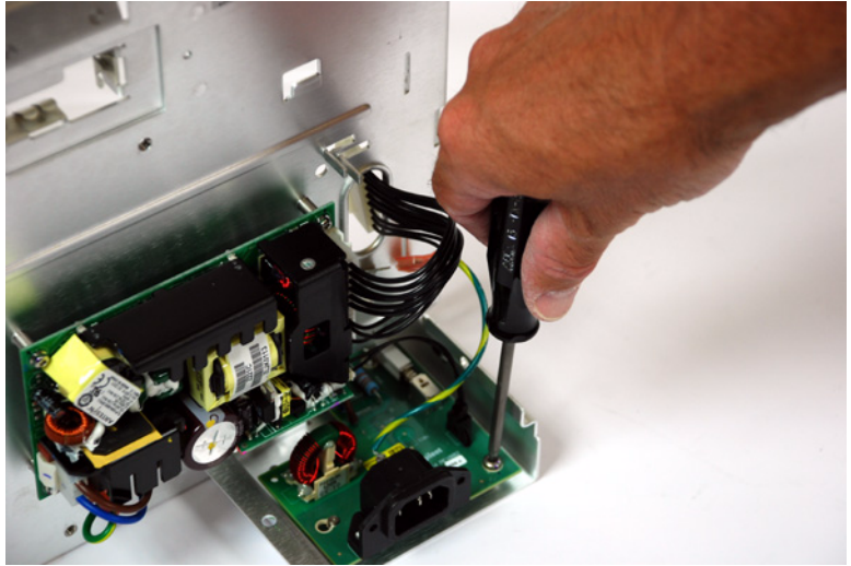
Figure 50 Removing the line filter board
